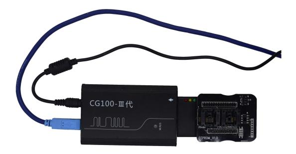
Enter the corresponding car model option to find the corresponding number, if dont have ,pls contact with manufacturer; if have, can remove chip directly and put into ATMEGA adapter
