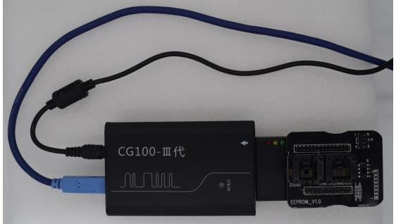
Can enter into corresponding car model select to find corresponding series number, If don't have ,pls contact technical support from manufacturer; If have, can remove chip directly to put into ATMEGA adapter Anise chips on the seat ,then reading and witting .
