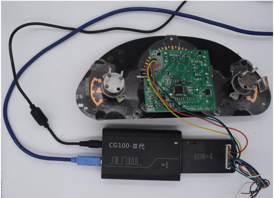
After connect line, check carefully, can connect power to operate after confirm without any mistake Software read out idiomatically mileage data, It show "save".
