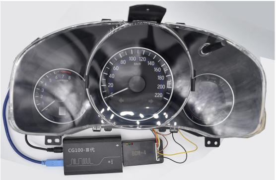
After connecting line, check carefully, only confirmed can be connected power to operate.
