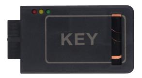
KEY adapter support all kinds of cars key to be matched for users with full version of CG100, providing freely KEY adaptor, which can be match CAS3 CAS3+ CAS4 CAS4+ calculate ISN code, analysi CAS data right or
