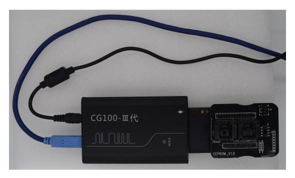
Enter the relative model options and find the corresponding number, if dont have, can consult technology of manufacturer: if have, can remove chip directly and put into anise chips of ATMEGA adapter, then, can read and write.
