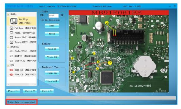
Mileage data finished writing, software provide instruments testing function, click "turn on power", check if correct or not.
