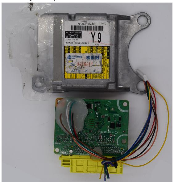
Enter the relative model options, find the corresponding airbag number, if not, you can consult the manufacturers of technology; if so, you can follow the wiring diagram of the software wiring, if the physical and software to provide the wiring diagram are different, can also follow the chip pin diagram Carry the scale wiring, pay attention to the number of pins to be consistent.
