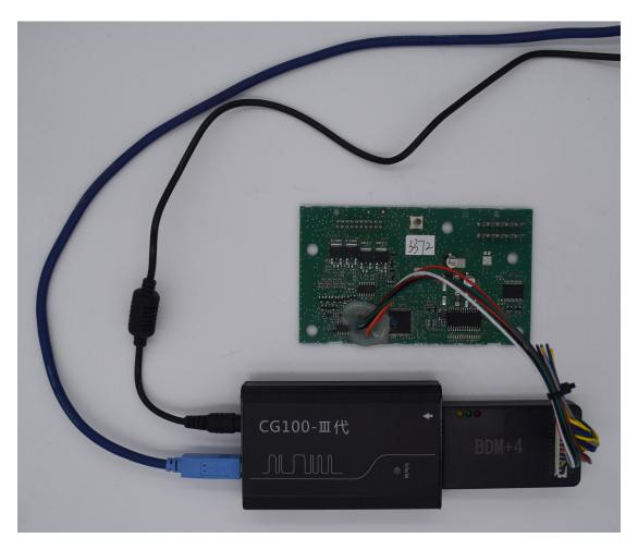
After connect wire, check carefully , only confirm can connected with power to operate.click "reading".
