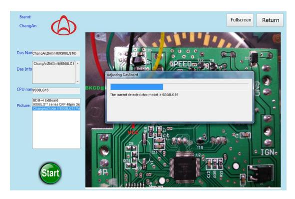
Save the original car data, the software will automatically analyze the mileage data.
