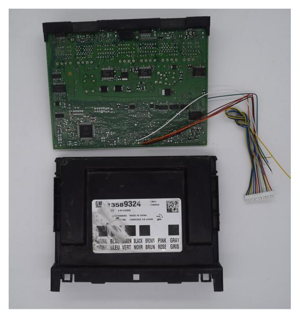
Enter the relative model options, find the corresponding BCM number, if not, you can consult the manufacturers of technology; if so, you can follow the wiring diagram of the software wiring, if the physical and software provided by the wiring diagram are different, can also follow the chip pin Carry the scale wiring, pay attention to the number of pins to be consistent.
