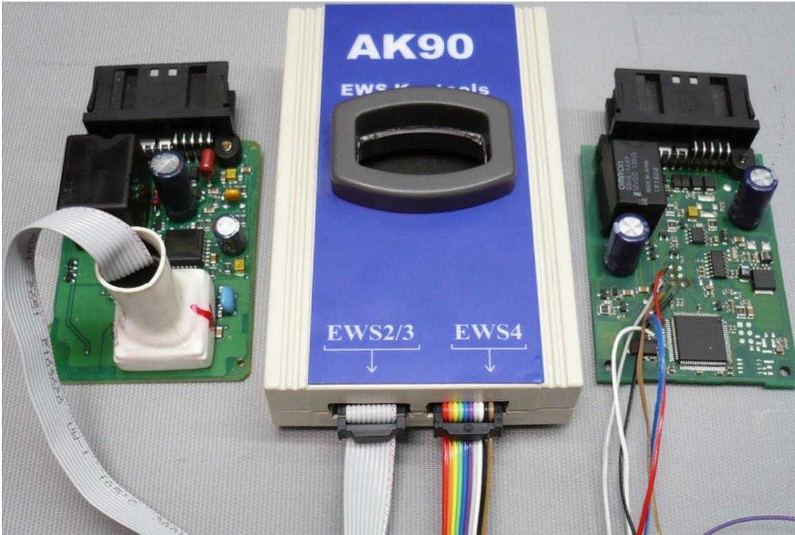
For EWS2,3 you have to clean the pins on the MCU for reading data .
