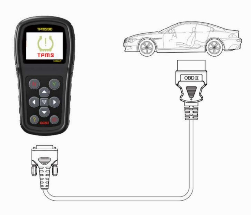
Turn off the ignition switch and connect TPMS90 to the vehicle diagnostic port through the OBD connector. You can perform operations such as sensor ID reading and writing.
