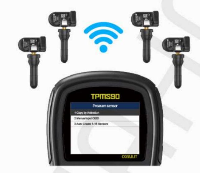
The sensor is placed in the TPMS detection area, the device is opened to select the corresponding vehicle type, and the sensor can be burned, identified, copied and other operations.
